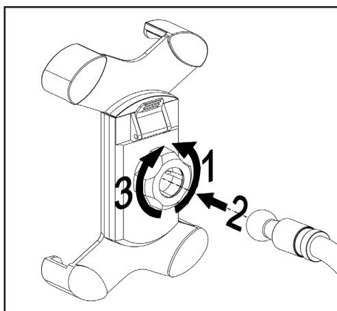
**1** Open the clamping nut on the smartphone holder in the UNLOCK direction until the swivel joint **2** snaps into the smartphone holder with slight pressure.
