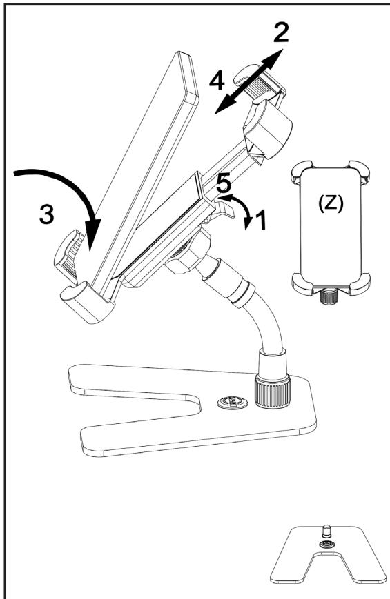
Open the clamping lever **1** on the smartphone holder, and slide the smartphone holder apart **2**. Lower the smartphone from above onto the lower retaining tabs **3**, and place the smartphone in the smartphone holder. Push the smartphone holder together **4**. Use the clamping lever to lock the closed smartphone holder **5**. Clamping lever audibly engages.
