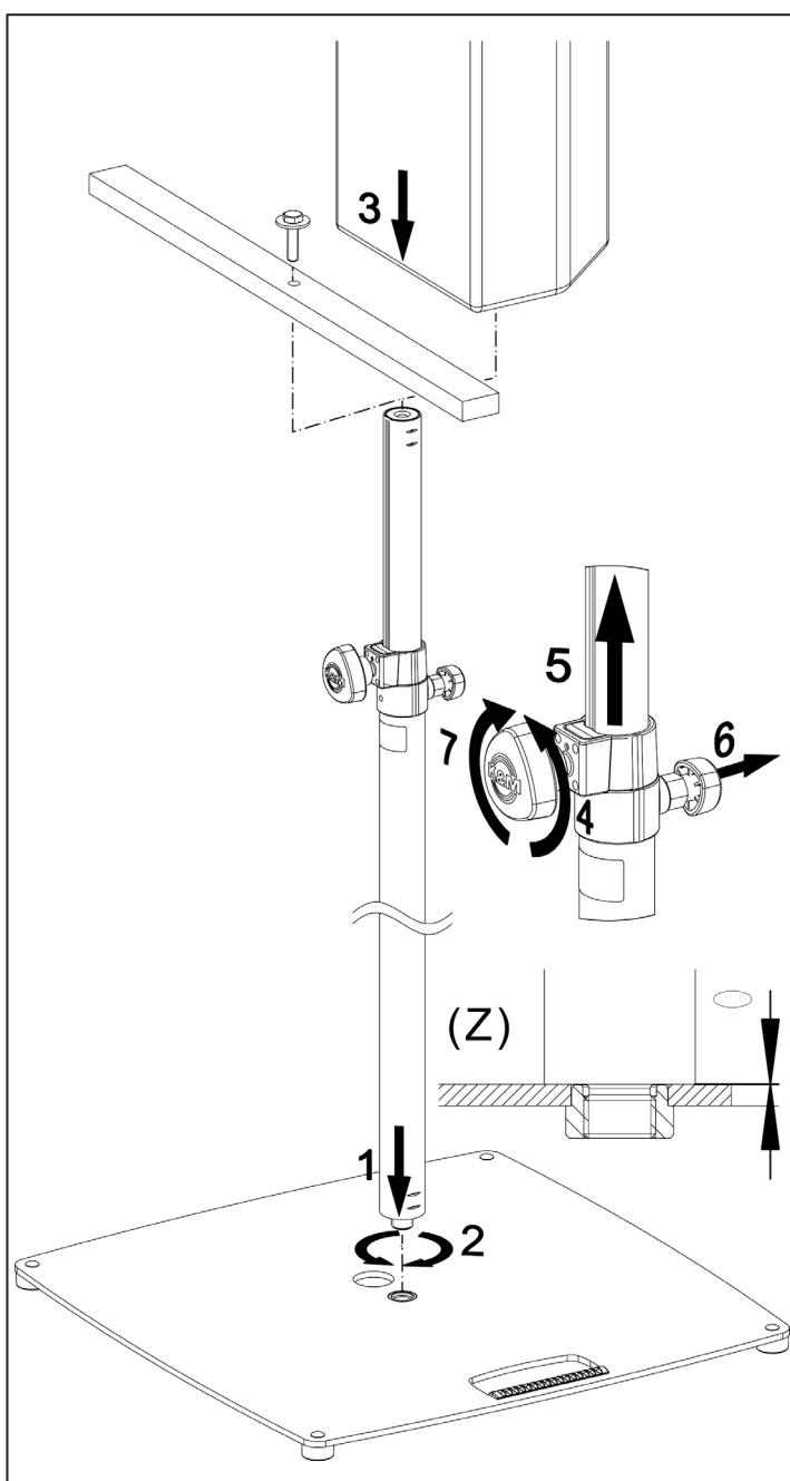
The locking screw must be screwed into the clamp once before first use.
