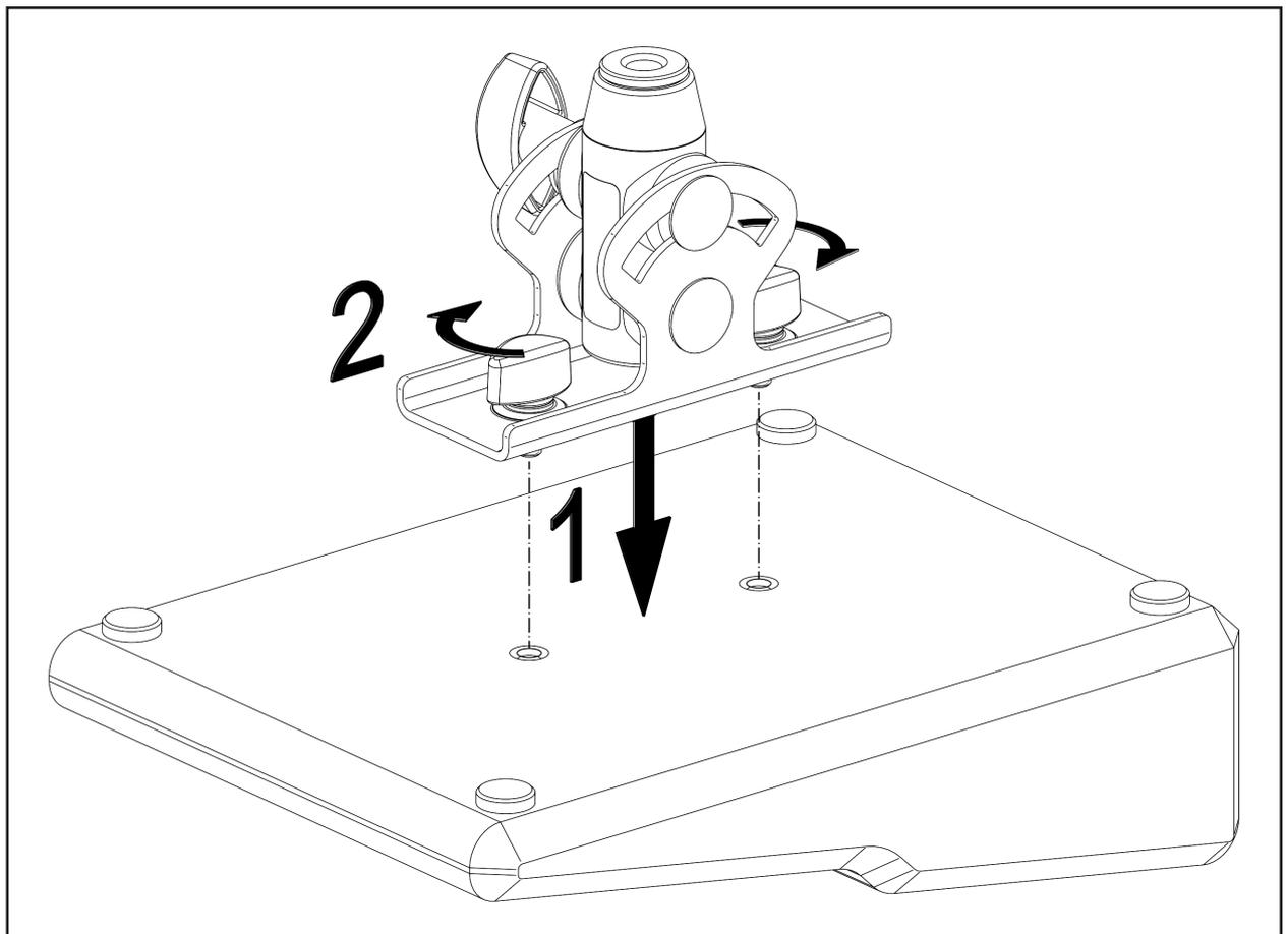
Place the equipment so that the mounting threads are pointing upwards. Attach the stand adapter **1**, and hand-tighten with the clamping screws **2**.
