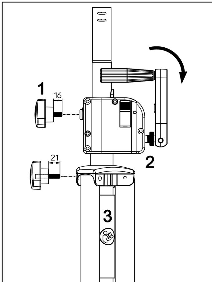
The clamping screws **1** must be screwed into the crankcase (M8 x 16 mm) and the foot clamp (M8 x 21 mm) once before first use.
