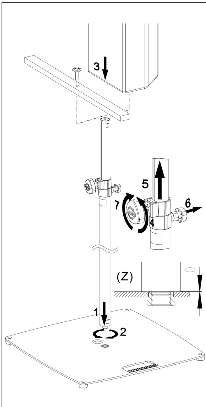
The locking screw must be screwed into the clamp once before first use.
